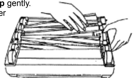
To reinsert the rotorblade, center it in its cavity and gently **press down** on the end until it snaps in place.
